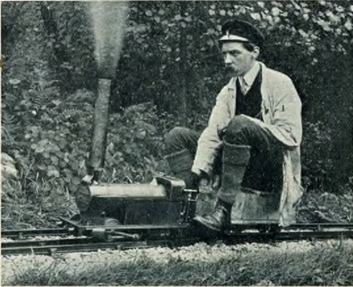
FIG. 1.—MR. G. S. MITCHELL'S 3\frac{1}{2} " GAUGE RECORD BREAKER. (3 miles non-stop with passenger; 1\frac{1}{4} miles non-stop with one firing.)
